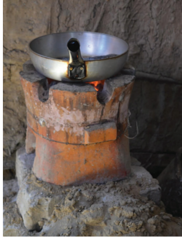
Figure 5.3: Photo of traditional charcoal cookstove used in the Tambogrande region of Peru.
